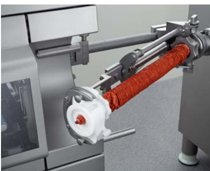
Casing brake assistant – semi-automatic casing brake holder system
