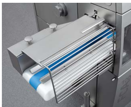
Fully hygienic conveyor belt, dismantling without tools
