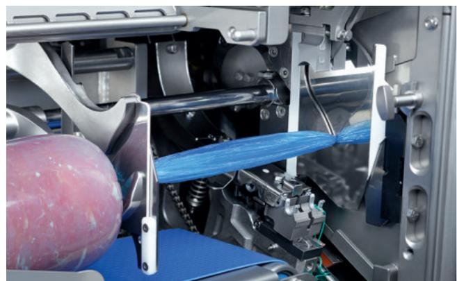
Fig. 3: The clipping machine has an overall spread of 300 mm for slack, air-free filling of moulded products.
